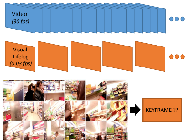
Fig. 1. Visualization of image obtained from video sequence and lifelogging devices. There are obvious differences in frame rate between both image domains. Noncontinuous image sequences are obtained from a lifelogging device. This kind of image sequence poses difficulty as far as event segmentation and keyframe selection using related features between consecutive frames are concerned.
