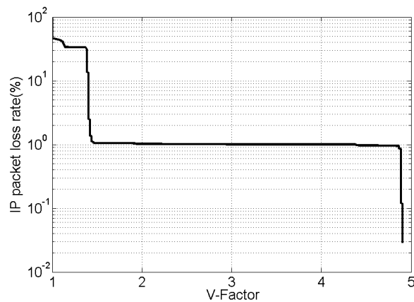
Figure 9. Relationship between the IP packet loss rate and V-Factor.
