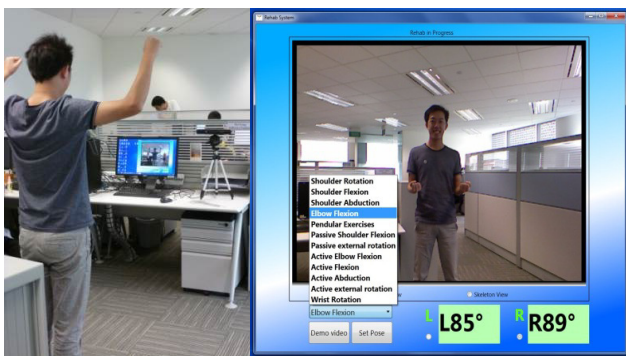
Figure 1. (a) (left) Pei performs a shoulder rotation while the assistant shows him the degree of rotation. (b)(middle) The screen reminds Pei how to do pendular exercises, while preparing to count his repetitions. (c)(right) The assistant's
